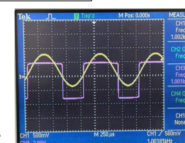
Above: Sine wave (yellow) digitized by Schmitt trigger (purple)
